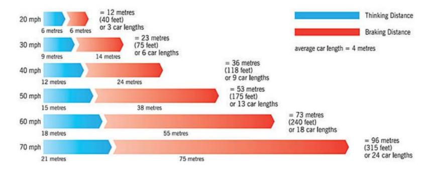
It takes 3 times the distance to stop at 60MPH as it does to stop at 30 MPH
